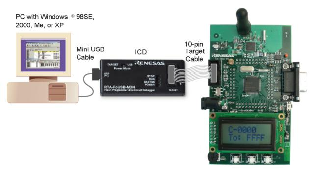
Figure 4-2 ZDK Development System Connectivity
